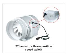
The double-speed motors are controlled with a built-in switch (V option) or an external switch for multi-speed fans (available upon separate order). An integrated speed controller (option R), an external TRIAC or autotransformer speed controller (available upon separate order) are used for smooth speed control when connected to the maximum speed terminal.
