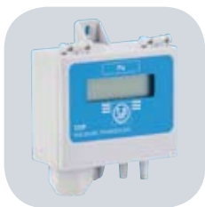
TDP-S / TDP-D Pressure sensor. Enables you to control the pressure in the fan inlet. Pressure range: 0-2500 Pa. Output signal: 0-10V/4-20 mA.
